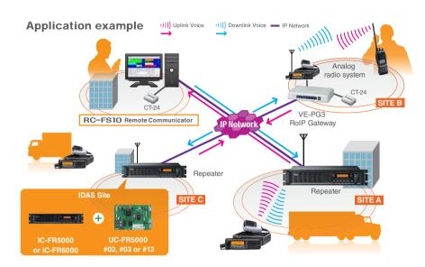
The RC-FS10 Remote Communicator creates an IP-based virtual radio on a Windows®-based PC, and works as a simple dispatch station to communicate with radio terminals. The RC-FS10 can be used with Type-D multi-site trunking, NXDN conventional. dPMR mode 2 radio systems, and an analog radio system through the VE-PG3.
